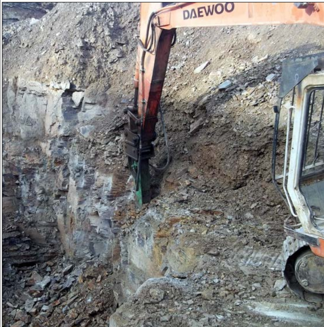
Plate A2/21: Second excavator using a 'pecker' attachment at second working face. Two faces are worked simultaneously to provide efficient operations.
